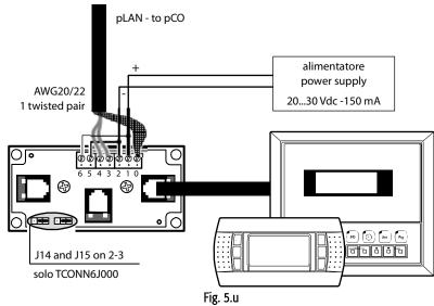
**A** Important: the overall length of the network must not exceed 500 m. Consequently if the terminal is also remote the length of the cable to the terminal is included in the calculation of the total length.
