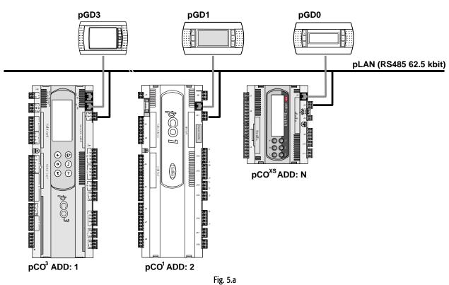
The standard communication speed over the network is 62500 bps but some devices also support speeds of 115200 bps.
