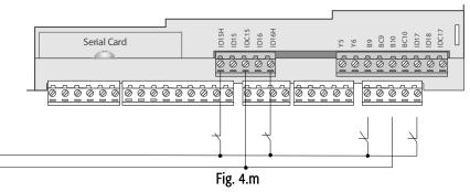
The uncertainty of the switching threshold ranges from 43 to 90 Vac. It is recommended to use a 100 mA fuse in series with the digital inputs.
