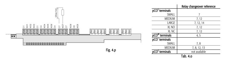
Warning: the load of the SSR relay is powered at 24Vac/Vdc, thus all the other terminals in the group, from 1 to 6, must be powered with the same tension due to the absence of double insulation within the group. Moreover, terminals from 1 to 6 can be powered at 110 to 230 Vac using a safety transformer (Class 2).
